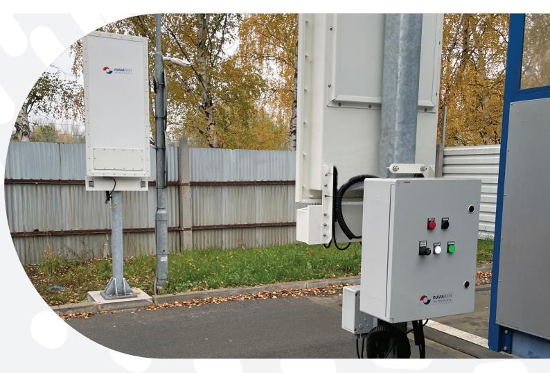
The detection gate is equipped with two 25 L scintillation detectors that can be used for quick and easy inspection of trucks and cars transporting scrap metal. The high sensitivity of the detection system ensures high reliability of detecting a potential source of ionising radiation.
