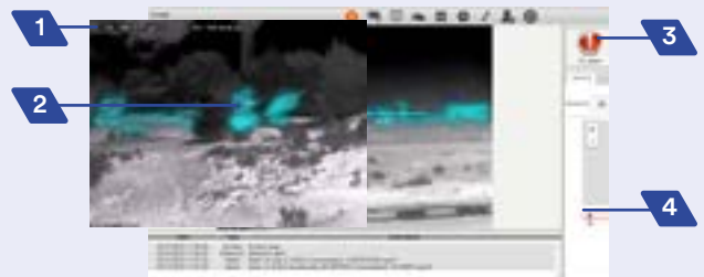
1 - Identification 3 - Alarm 2 - Gas cloud 4 - Gas list
