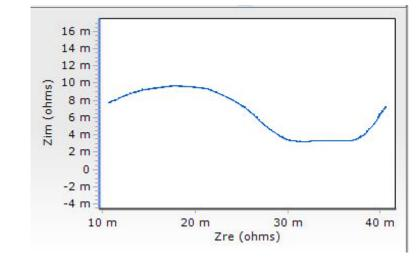
Galvanostatic EIS test at 7 Amps (RMS) signal on same commercial Li-ion battery pack. Data represented as Nyquist plot.
