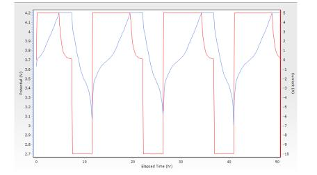
PMC-1000 with PMC Booster for charge-discharge (CC-CV action) tests on a commercial Li-ion battery pack. Charge at +5 Amps followed by Voltage Hold (until current decays to 100 mA); followed by discharge at -10 Amps.
