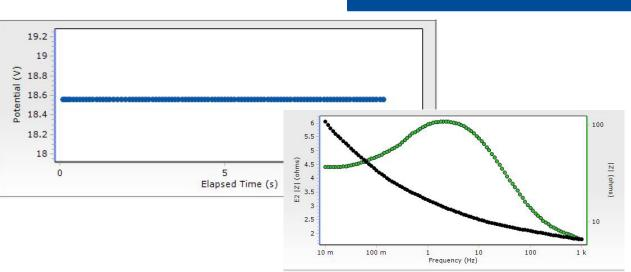
Using the 6-WIRE function of the PMC-2000A, a single Potentiostatic EIS experiment simultaneously measures the impedance of a single battery (black, 2-6 Ohms) and 2-battery stack (green, 10-100 Ohms) of 9 Volt commercial batteries. Even without a booster or option, the PMC-2000A determines one of these batteries dominates the impedance of the stack, while still producing 18 V DC.
