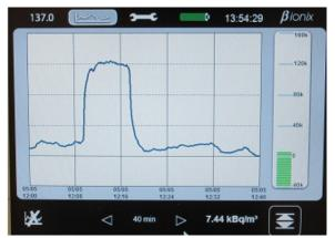
Example of the response at 100 kBq/m³ **B IONIX 3 – MES**Volumetric activity measured
