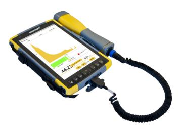
The RayMon10® is the highest resolution CZT handheld radiation monitor in the world. It can be used to detect, measure, identify and analyse gamma ray emitting radionuclides. The CZT detector produces high resolution gamma-ray spectra for clear and unambiguous interpretation. The RayMon10® algorithms provide spectral dose, radionuclide identification, line analysis and activity quantification.
