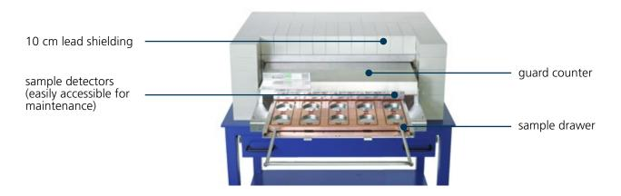
The special design of the Berthold Low-Level counters eliminates not only the ambient radiation, but also eliminates the influence of cosmic radiation.
